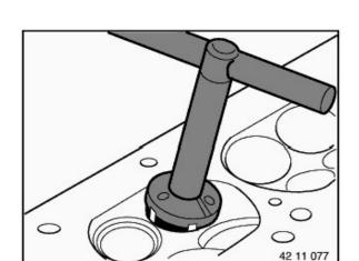
Machine valve seat surface with special tool 00 3 520 or with 00 3 580 in accordance with tool manufacturer's instructions.
