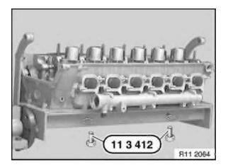
Secure cylinder head to special tool 11 1 065.
