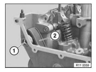
Release bearing pin (1) for tensioning rail (2).
