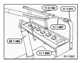
Provide special tools for removing valve springs.
