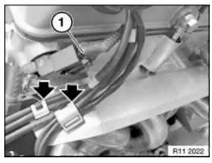
Disconnect plug connection (1) on sensor of exhaust camshaft.
