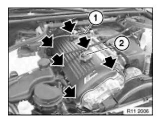
Remove hose (1) for engine vent.
