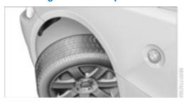
To gain access to the headlamp covers, turn the front wheels in the required direction.
