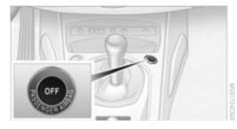
The system checks that the airbag system is functioning properly when the ignition key is turned, and the indicator lamp in the central console lights up for several seconds.
