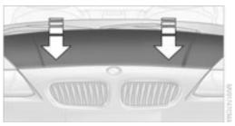
Allow the hood to fall from a low height and push on both sides so that it audibly engages.
