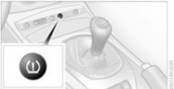
Initialize the system only when the inflation pressure has been corrected or modified, e.g. if a tire was changed.
