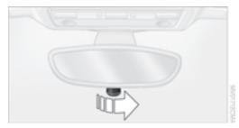
To reduce the glare from vehicles behind you when driving at night, turn the rotary knob.
