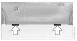
The jacking points are located at the positions indicated in the illustration.
