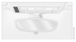
In vehicles that are wired for a telephone\*, the cover of the hands-free microphone is located in the headliner close to the interior lamps.
