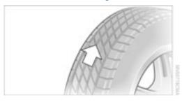
Inspect your tires frequently for tread wear, signs of damage and for foreign objects lodged in the tread. Check the tread depth.
