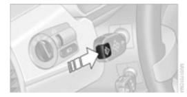
With the ignition key in position 1 or higher, you can use the button in the turn signal lever to retrieve information from the computer for display in the instrument cluster. Every time you press the button briefly in the direction of the steering column, a new function is called up for display.
