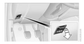
The Onboard Diagnostic OBD interface socket is located on the left of the driver's side behind a specially marked cover located beneath the instrument panel. The cover has the letters OBD on it.
