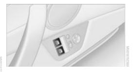
The illustration shows the power window switches in the trim of the passenger door.
