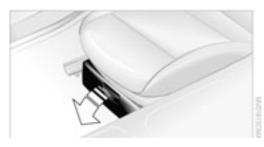
The first-aid kit is located beneath the passenger seat.
