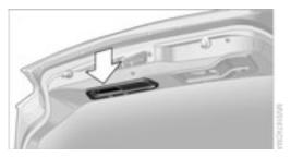
The handle recess in the interior trim panel of the luggage compartment lid makes it easier to pull the lid down.
