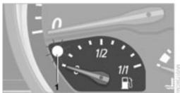
Once indicator lamp 1 stays on continuously, there are still approx. 2 gallons / 8 liters of fuel in the fuel tank.
