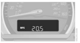
If you continue to press the button on the turn signal lever, the average fuel consumption last displayed is recalculated from that point in time.
