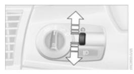
Turn the rotary dial to adjust the illumination intensity.
