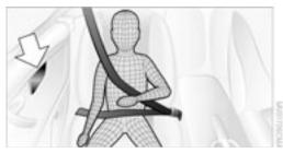
This is the correct way a larger child no longer using a child-restraint system should sit wearing the safety belt, when the airbag system is activated.
