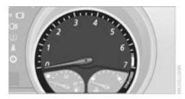
Never allow the engine to operate with the needle in the red overspeed sector of the gauge.
