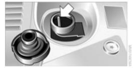
Correct coolant level when the engine is cold – at approx.  $68 \, ^{\circ}\text{F} / 20 \, ^{\circ}\text{C}$ :
