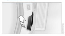
Pull the lever located under the left-hand side of the instrument panel.
