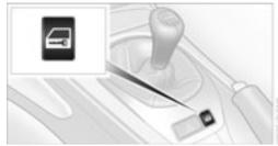
You can use this button to control the central locking system whenever the doors are closed. The doors and luggage compartment lid are unlocked or locked only. The anti-theft system is not activated.
