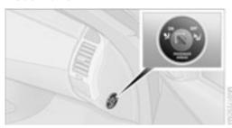
Deactivation of the passenger airbags system deactivates the passenger front, knee and side airbag. The airbags on the driver side remain active.
