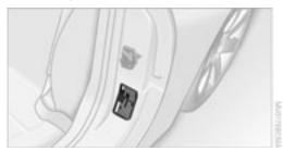
The specified inflation pressures are provided on a sticker attached to the B-pillar and are visible when the driver's door is open.
