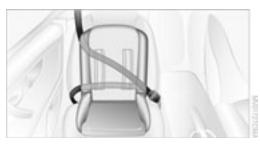
Commercially available child seats complying with the legal standard are designed to be secured with a seat belt or with the seat belt portion of a combination lap/shoulder belt.
