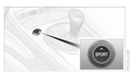
The Drivelogic feature lets you select between the standard and sport program. The sport program is recommended for performance-oriented driving.
