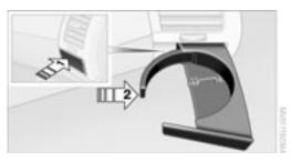
Beverage holders are located on each side beneath the air outlets.
