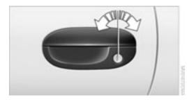
One turn of the key in the driver's door lock to unlock the driver's door only and the fuel gas door.
