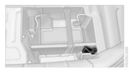
The onboard tool kit is stored in a tool pouch. It is located in the luggage compartment beneath the floor panel.
