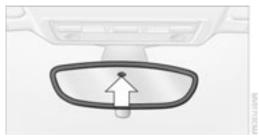
This mirror automatically dims through an infinitely variable range and switches automatically to its clear, undimmed mode whenever you engage reverse gear or place the selector lever in position R.
