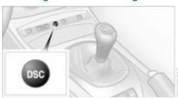
Press the DSC button briefly. The DTC indicator lamp comes on and stays on.
