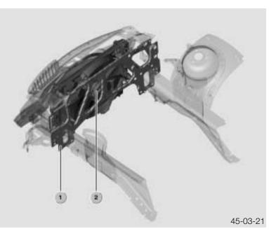
**Cooling Module in Installation Position**
