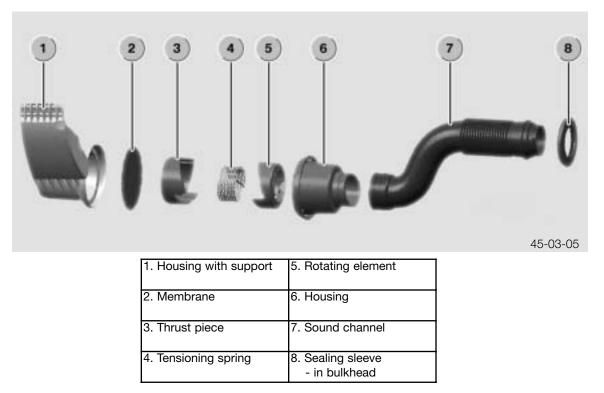
The sound generator is connected by a membrane (2) to the column of air in the intake manifold. The pressure pulse is transmitted into the passenger compartment via this membrane, which also ensures a "sealed" intake system.
