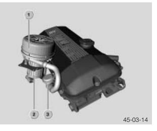
The electrically driven secondary air pump is mounted to the body in the engine compartment (in the area of the right-hand strut tower). To draw in secondary air, the SLP has an integrated air filter element. The air filter element is maintenance-free during the service life of the vehicle.
