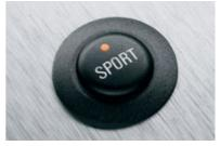
Driving Dynamic Control (sport mode), at the touch of a button, engine response to the accelerator becomes even more spontaneous. With the automatic gearbox, the sport program is engaged and gear shifts occur faster. Steering assistance is also reduced for improved feel of the road, and cruise control accelerates faster (standard on the Z4 2.5si and Z4 3.0si¹).
