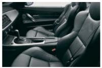
☐ M sports seats for driver and front passenger, sporty design with integrated headrests; optimum lateral support in dynamic driving situations provided by highlycontoured seat sides; wide range of longitudinal settings; individual adjustment for seat height, thigh support and seat angle.
