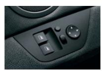
■ Electric window lifts incl. comfort control also controlled by the key by pressing and holding the central locking button on the key when locking the vehicle, open windows automatically close.
