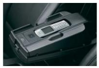
☐ Preparation for mobile telephone with Bluetooth interface, incl. hands-free installation, charger connection and antenna. Snap-in adapter (Original BMW Accessory) connects a Bluetooth mobile phone, which can be operated, for example, via the multifunction steering wheel. Your BMW partner will be happy to inform you about recommended telephones.
