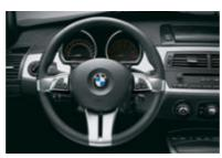
☐ Multifunction sports leather steering wheel, control of radio and telephone (optional) via integrated buttons.
