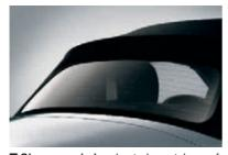
■ Glass rear window, heated; scratch-proof rear window ensures optimal back vision at all times.
