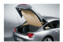
■ Comfort opening: the luggage compartment cover opens in unison with the tailgate when in its extended position, for convenient access.
