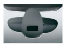
□ Rain sensor incl. automatic headlight control: when activated, the rain sensor automatically turns the wipers on and adjusts the wiper frequency according to the intensity of the rain. The headlights are automatically activated on dipped beam when daylight fades or when entering a tunnel.
