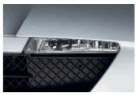
☐ Fog lights integrated into the front air dam. The foglamps provide extra safety in bad weather conditions (including heated exterior mirrors and front screenwasher nozzles).
