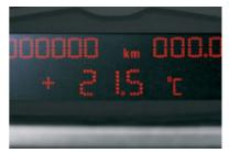
□ On-board computer provides data on average speed, average fuel consumption, range, time and outside temperature (standard on the Z4 2.5i, Z4 2.5si and Z4 3.0si¹).
