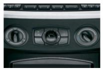
☐ Air conditioning, including microfilter, ensures comfortable climate conditions in the vehicle interior at any time of the year, with manual adjustment of air volume and air distribution. (Standard on Z4 2.5i, Z4 2.5si and Z4 3.0si²).
