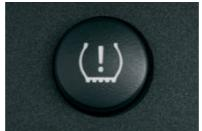
■ Runflat Indicator detects drops in tyre pressure and warns the driver with an indicator light in the instrument panel. Should pressure drop dramatically over a short period, the driver is warned by an additional acoustic signal.0
