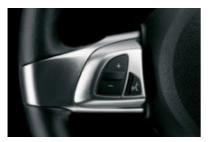
□ Voice control system for navigation system Professional. Voice computer can be activated at a press of a button on the sports leather steering wheel with multifunction, and telephone or navigation system can be controlled via voice direction.
