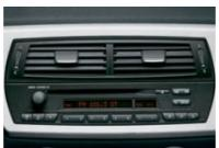
□ Radio BMW Business CD, 4 x 25 watt power output, antenna diversity, integrated CD drive, motorised CD insert/eject, incl. MP3-decoder. Connection for BMW CD changer.
