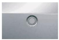
☐ Park Distance Control (PDC) for the rear area; facilitates parking and manoeuvring in tight spaces. The distance between your car and any obstacle is indicated acoustically.
