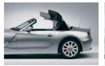
■ Manual roof operation, central lock for single-handed operation; thanks to the special folding mechanism no canopy or top lid is needed.
