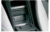
□ CD changer, incl. MP3 decoder, integrated into the storage compartment. The CD changer can hold up to six CDs (picture shows CD drive in combination with navigation system).
