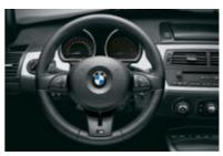
☐ M leather steering wheel with multifunction, thick contoured rim for superb grip. Integral buttons for radio, CD player and telephone (optional) control.
