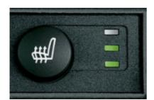
☐ Seat heating for driver and front passenger ensures a pleasantly warm seat surface within minutes (three settings) (standard on Z4 3.0si¹).
