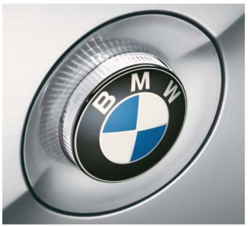
■ Side indicator lights with white lenses. When flashing, the light radiates outward from behind BMW's signature roundel.
