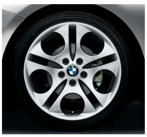
$\square$  Z4 Roadster 3.0i Sport Package with Ellipsoid (Styling 107) cast-alloy wheels, 18 x 8.0 front, 18 x 8.5 rear; and 225/40R-18 front, 255/35R-18 rear run-flat performance tires.<sup>2</sup>
