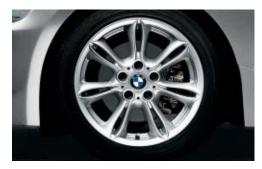
■ Z4 Roadster 3.0i with 17 x 8.0 Twin Spoke (Styling 103) cast-alloy wheels and 225/45R-17 run-flat performance tires.<sup>2</sup>
