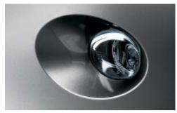
■ Ellipsoid, halogen free-form foglights are neatly integrated into the front bumper, uniformly illuminating the road ahead in bad weather.
