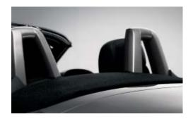
■ Rollover Protection Bars behind the headrests, as well as sheet-tube-reinforced windshield pillars, help provide excellent protection in the event of a rollover.
