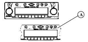
The volume is limited to a maximum value after the display has been folded down. After 20 seconds an audible signal indicates that the control component is folded down. The unit then switches off automatically.
