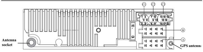
**Warning!** Terminal 30 and terminal 15 must always be connected separately, otherwise excessive current consumption occurs when the unit is switched off. Connection socket A is not the same for all vehicle types. Therefore, always measure voltages before installation.
